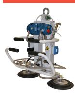
GP electric vacuum lifters are specifically designed for horizontal transferring of glass plates. GP...RB are also for manual rotation or swivel.
